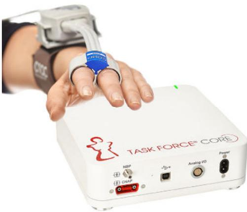
The Task Force® CORE measures continuous blood pressure and hemodynamics completely non-invasively and in real-time and is the state-of-the-art successor of the former Task Force® Monitor generation. Whenever continuous cardiovascular assessment is necessary, intermittent tools are insufficient and continuous invasive methods are not indicated, the Task Force CORE is the device of choice.
